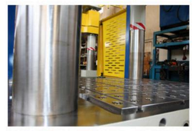
Press table complete with retractable spheres to facilitate loading and handling molds
